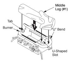
Figure 29 - Installing Middle Log (#1) (Base may very from illustration)
